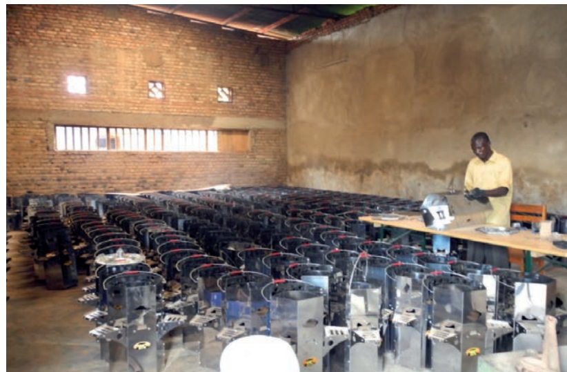
Assembly of the Save80 stoves in Rwanda.
