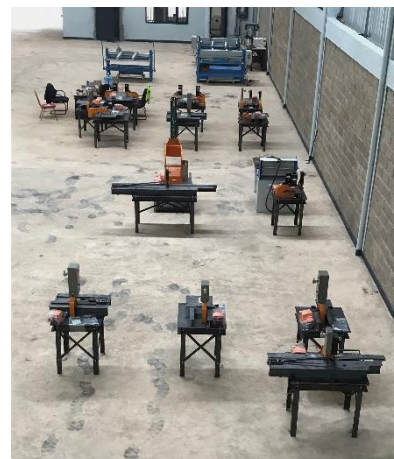
Shears and punching machines for the Kigali „Save80” production. Esp. the punching machines are tailor-made and in-house built for optimized workflow and product quality.
