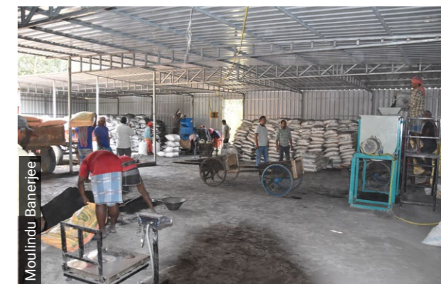
Hustle and bustle in our Kaukepara facility. Biochar is first crushed (blue machine in the background), then mixed with compost using a power mixer (right) and then filled into bags (front left)
