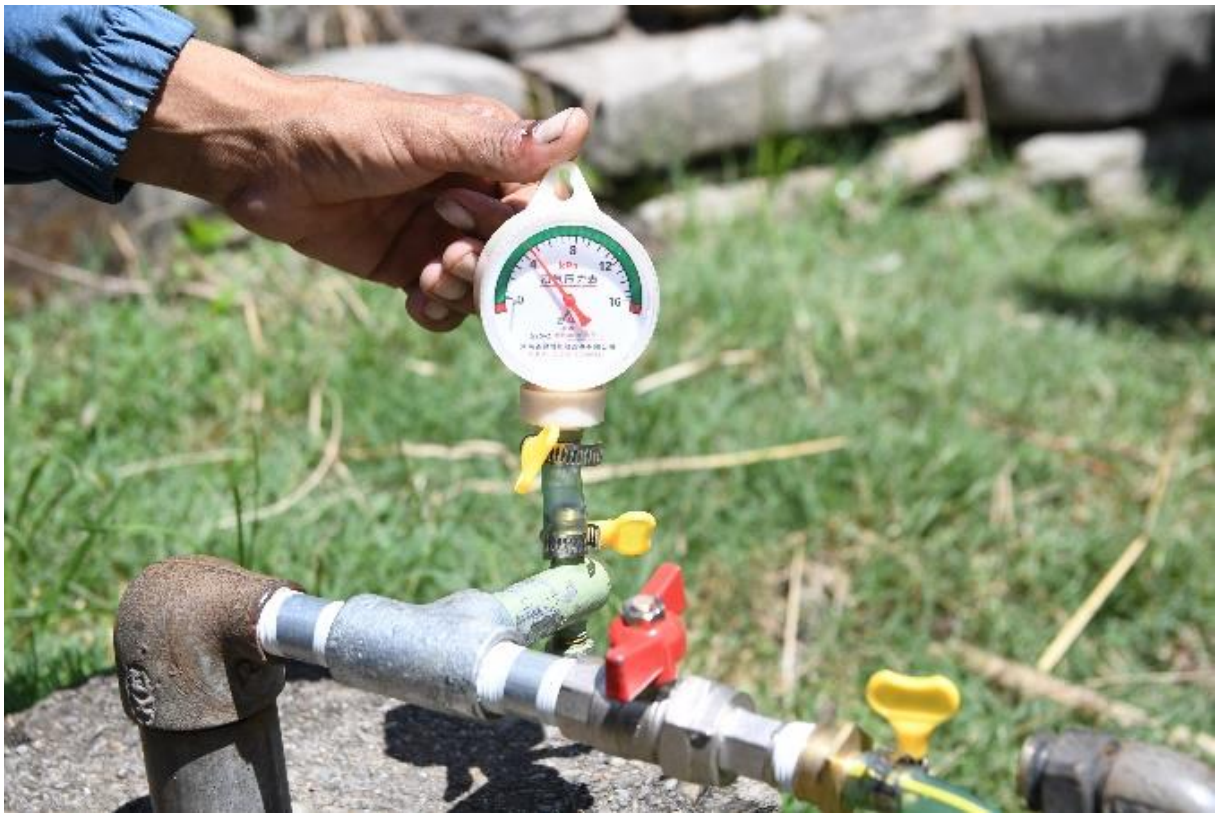
Picture 10: NBPA technician checks the tightness of the pipework system
